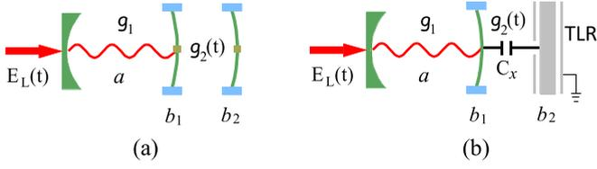
FIG. 1. Schematic representation of the system. An optical cavity mode  $a$  driven by a two-tone laser  $E_L(t)$  is coupled to an intermediate mechanical mode  $b_1$  with single-photon optomechanical coupling strength  $g_1$ .  $b_1$  is in turn coupled, with a time-dependent coupling strength  $g_2(t)$ , to (a) another mechanical oscillator, or alternatively (b) a transmission line resonator  $b_2$ .
